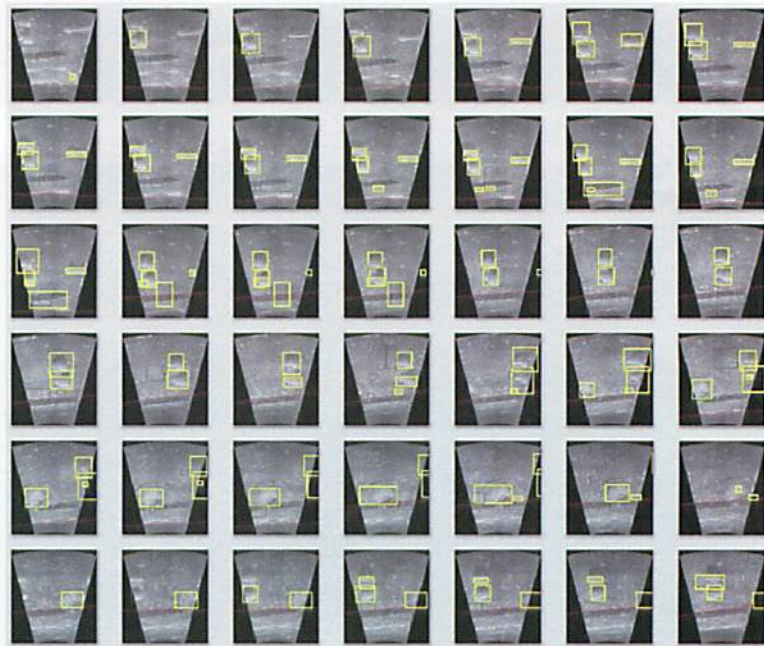
Figure 3: Automatic target recognition (ATR) results for a sequence of sonar frames containing regions of the hull inspected by the vehicle. Yellow boxes signify possible targets on the hull.
