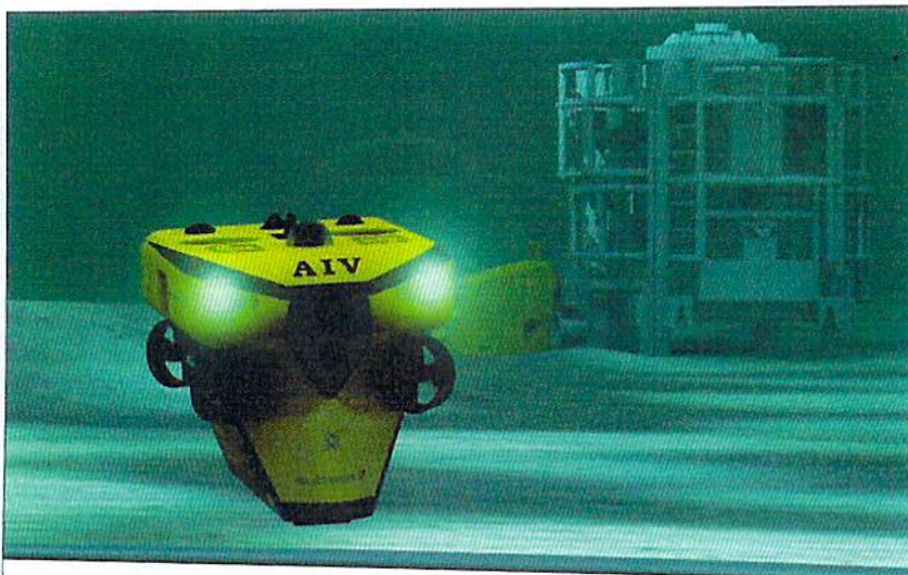
The autonomous inspection vehicle
